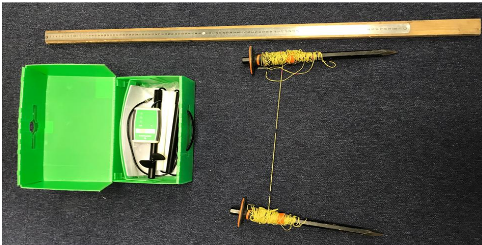
Figure 1: Example of LAWPRO equipment for flow measurements: budget flow metre, metre stick and builders' line with increments and fence poles.
