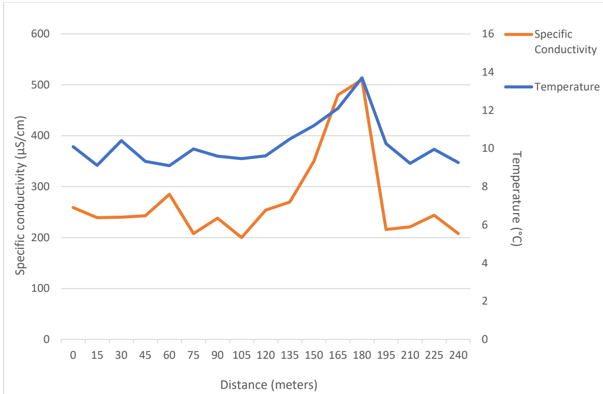
Figure 12: Specific conductivity and temperature profile over 240 metres stretch of stream.
