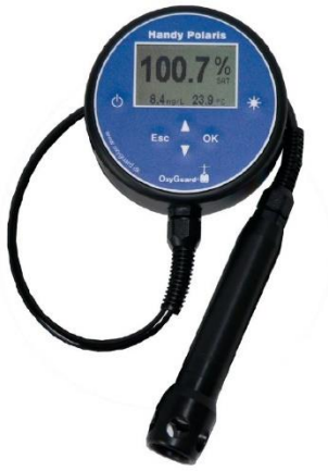
Figure 3-1: Example of a hand-held probe for spot measurements (OxyGuard Handy Polaris, which measures temperature and dissolved oxygen).
