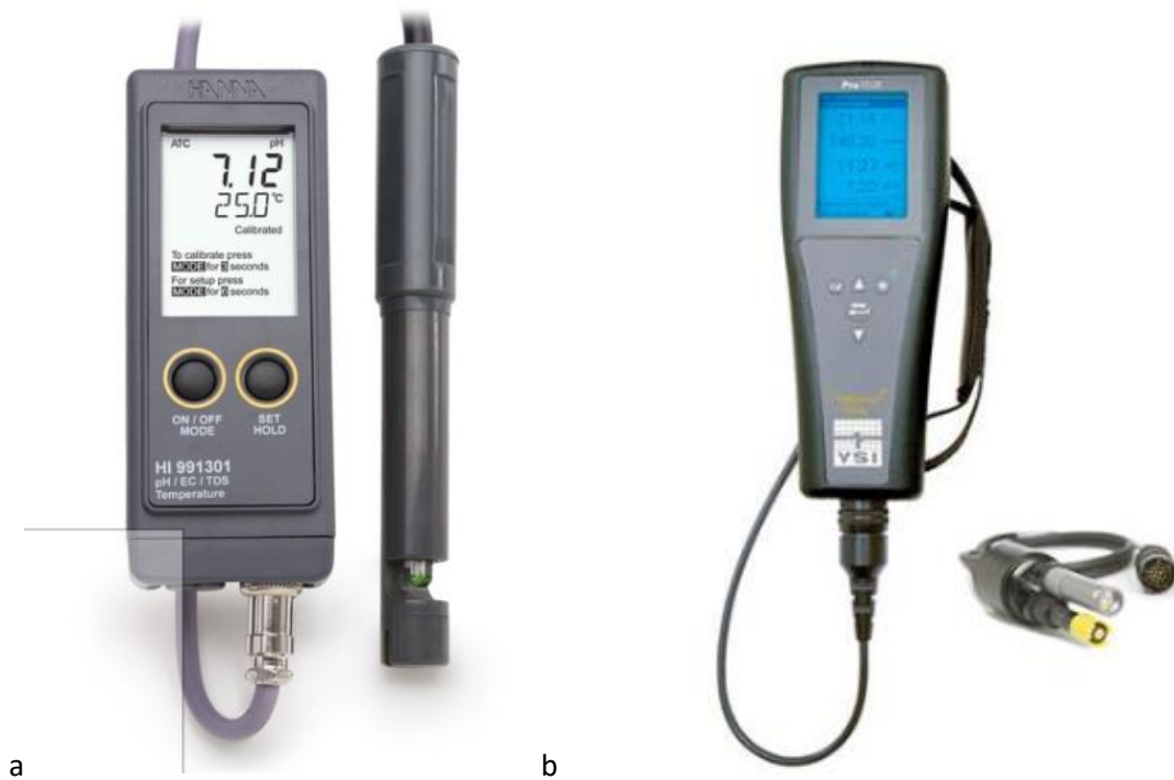
Figure 3-2: Example of more advanced probes for continuous measurements: a) Hanna (combined temperature and pH); b) YSi (pH, temperature, oxygen redox potential, dissolved oxygen, electrical conductivity, with case and cable for downloads, etc).
