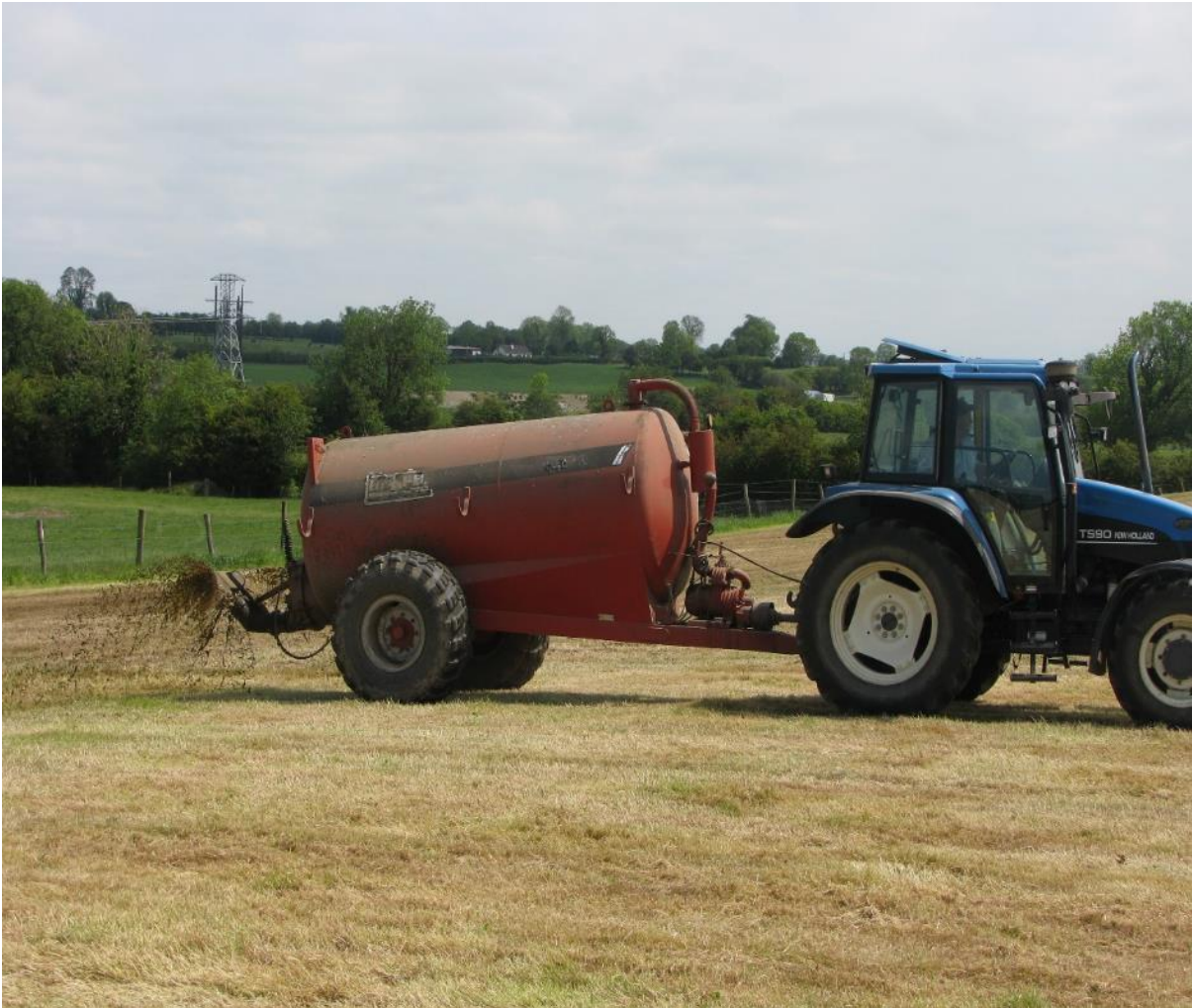
Figure 2-34: Standard vacuum tanker spreading by broadcasting through a pipe and a downward facing splash plate (Photo: Donal Daly).
