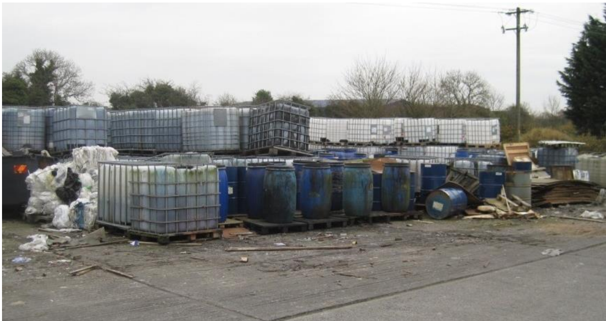
Figure 11-7: Waste materials and IBCs stored at rear of industrial facility in a haphazard manner – an indication of poor environmental management at a site creating a risk to waters (Photo: Emmet Conboy).
