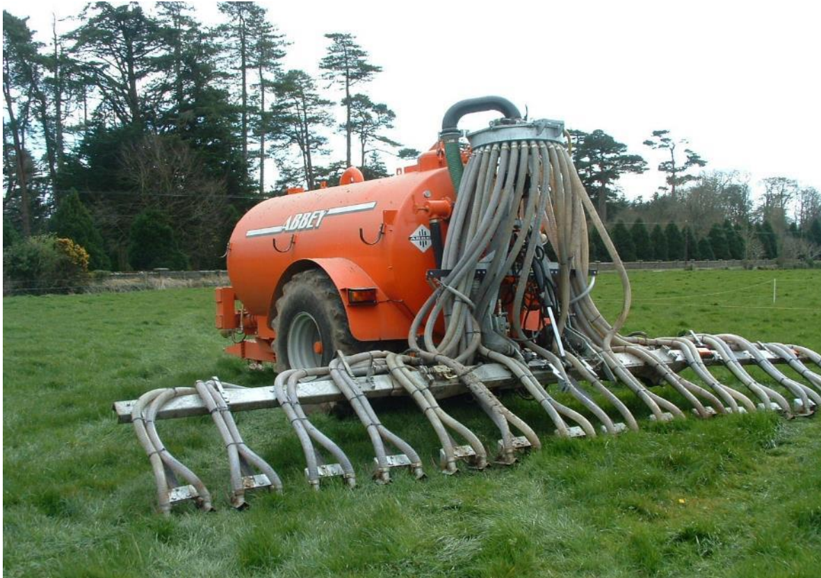
Figure 2-36: Band spreader/trailing shoe operating off a large vacuum tanker (Photo: Donal Daly).
