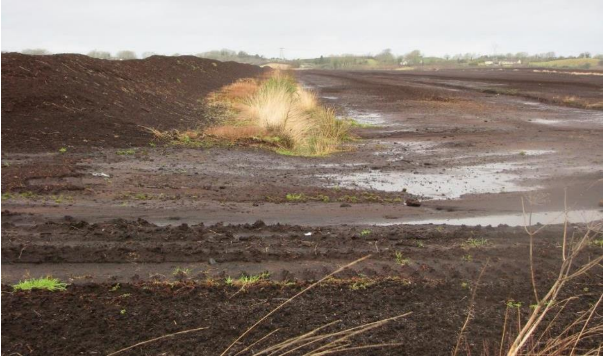
Figure 8-1: Mechanised peat extraction, with rows of milled peat and regularly spaced drains lowering the water table in the peat (Photo: Donal Daly).
