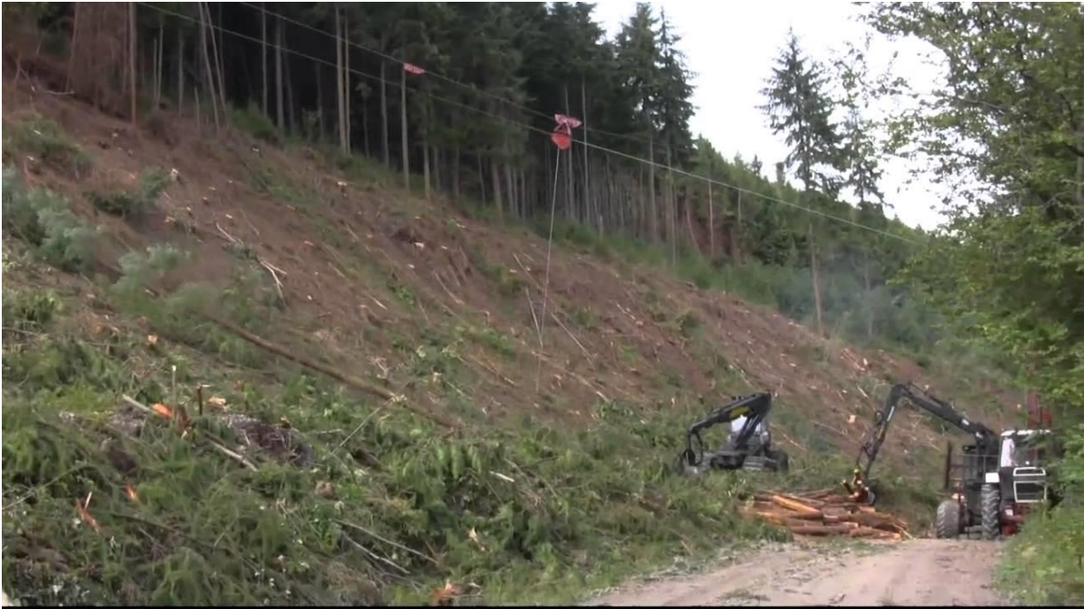
Figure 7-11: Cable extraction Wicklow. (Photo: Forest Service, DAFM)
