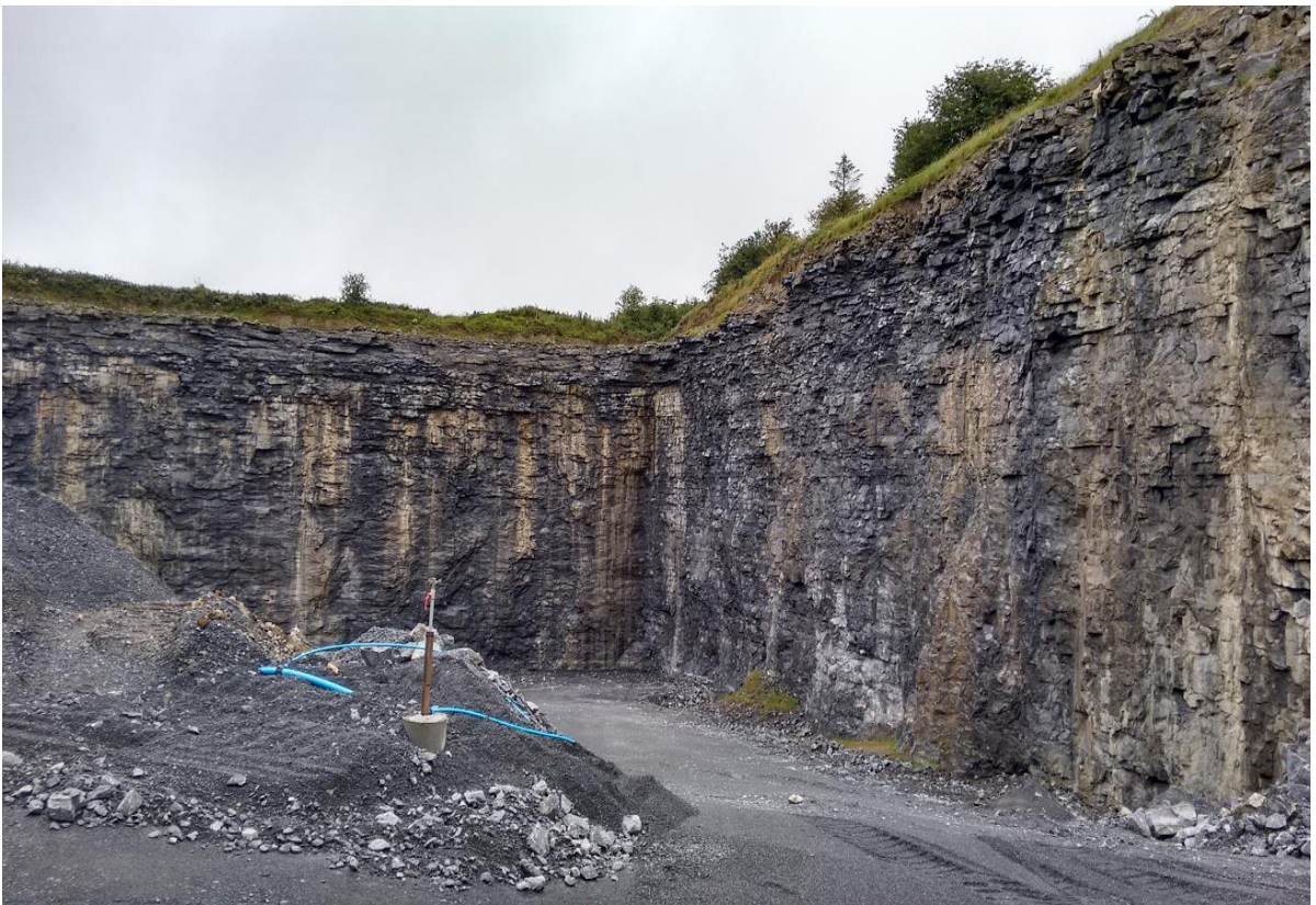
Figure 5-5: Seeps at base of epikarst 1 in quarry (shown by orange-beige streaks) (Photo: GW3D/GSI).
