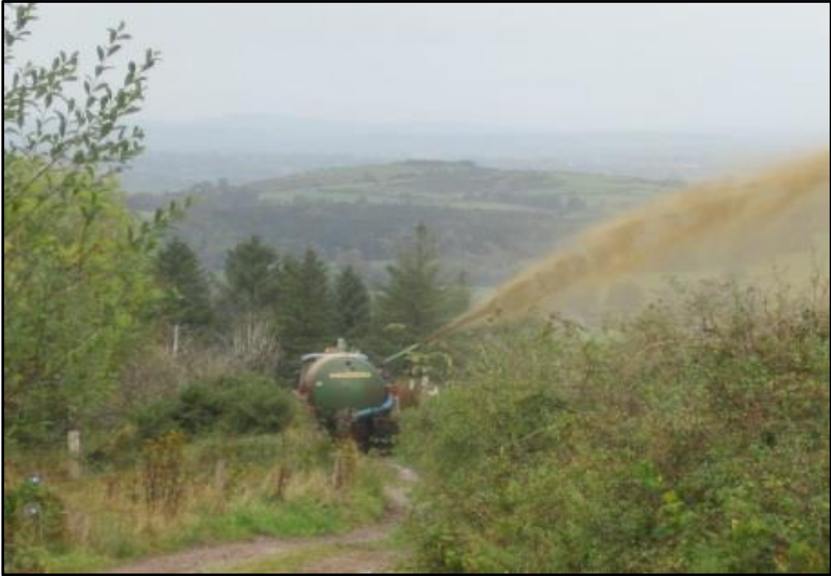
Figure 2-35: A vacuum tanker with a high level nozzle is pumping slurry onto ground that is often water logged due to heavy soil with resulting ground conditions that are unsuitable for the tractor to travel on the land. This is not acceptable practice (Photo: Andrew Holmes).
