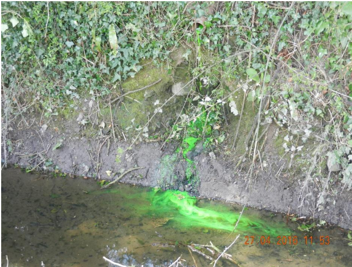
Figure 6-5: Bad Practice – Discharge of partially treated effluent from treatment system (Photo: Joan Martin).
